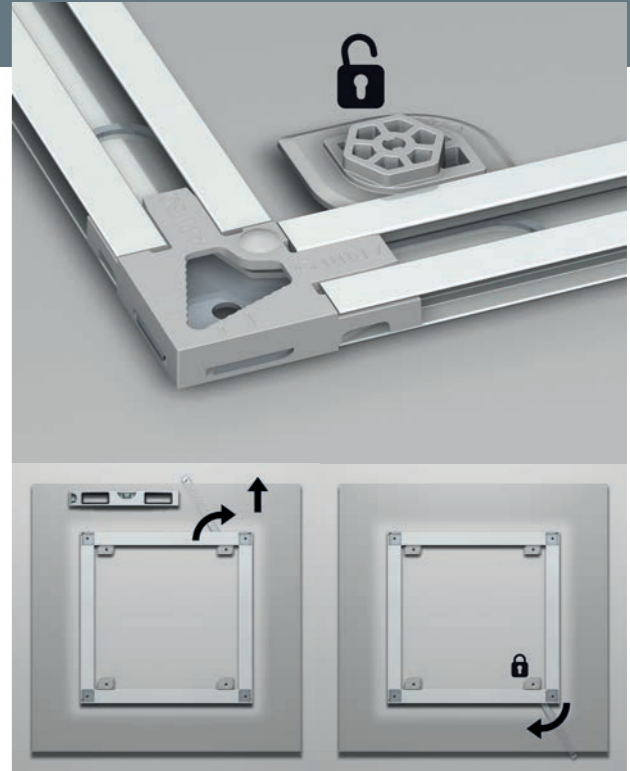
The panel can be fixed and secured to the wall using 4 Back Frame Security Clips. The frame hangs from the upper two Security Clips and the two lower Clips, once rotated using the Security Key, lock the frame into place.
